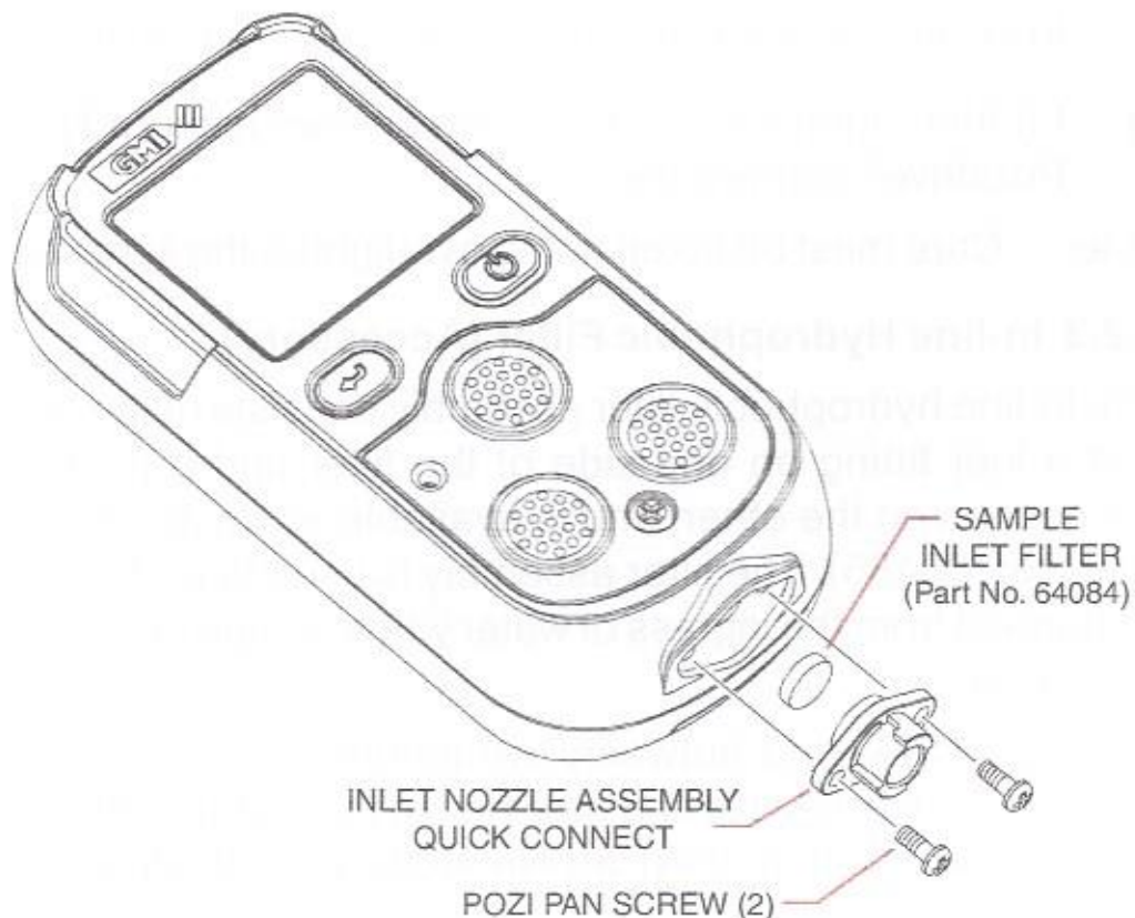
Fig. 5-2 Replace Inlet Filter
