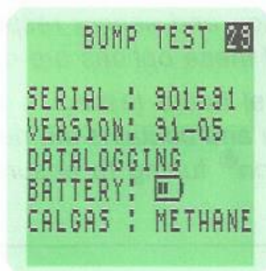
Fig. 3.1 Bump Test mode
