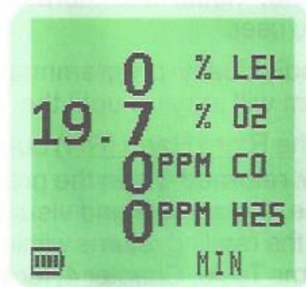
Fig. 2-20 Minimum Gas Values
