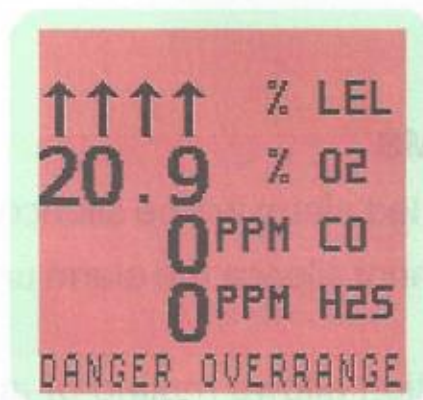
Fig. 4-3 Over Range Alarm
