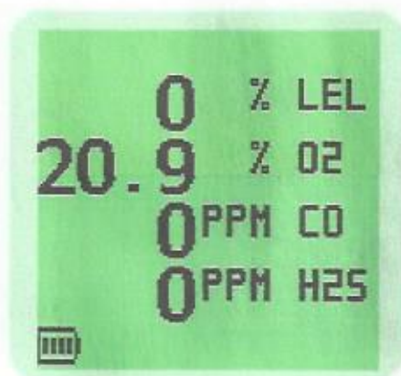
Fig. 2-18 Normal Operating Display
